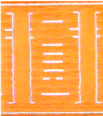
Figure 2. Buried Via 14-Layer Resin Filling Utilizing Laser-Drillable LD Materials (Layer 1-2 and 13-14 fabricated with LD Technology).
