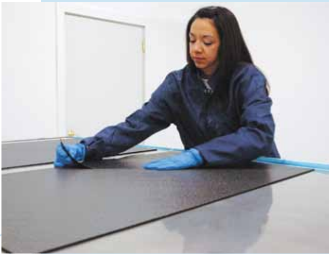
Initial lay-up of flat panels for a military aerospace structure. Panels are subsequently machined after curing.
