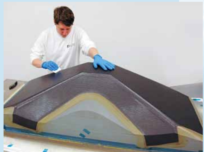
Space vehicle structure. Prepreg is "laid up" on a tool prior to curing.
