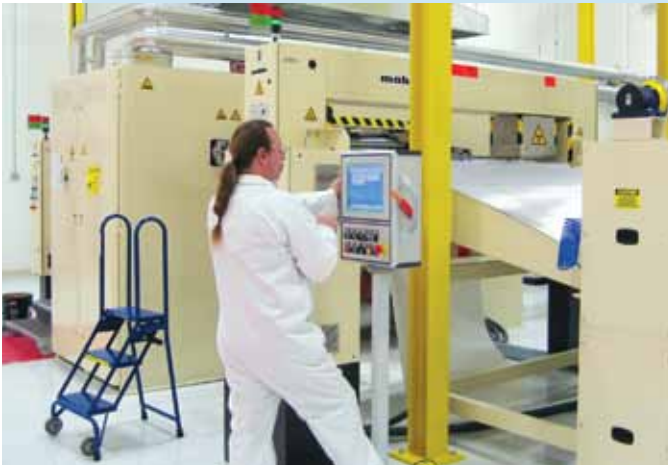
PATC's hot melt line is capable of producing unitape and prepreg up to 60 inches in width.
