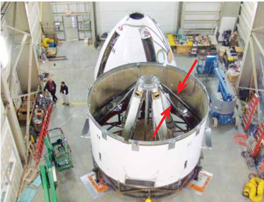
Park’s patented composite struts on NASA’s Max Launch Abort System (“MLAS”) test vehicle. The struts indicated by the arrows above are 11 feet in length.
